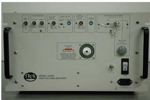
Figure 7. High voltage amplifier (Trek,model5/80A).
