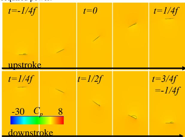
**Figure 3 Pressure coefficient distribution around the required power minimum flapping motion.**
