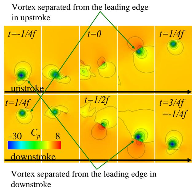
**Figure 1 Pressure coefficient distribution around the thrust maximum flapping motion.**
