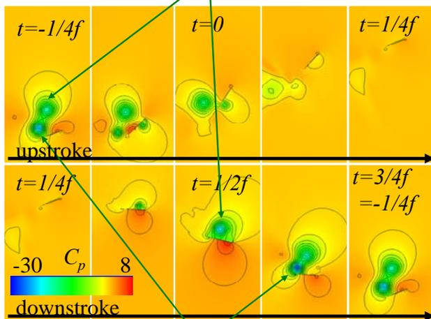
**Figure 2 Pressure coefficient distribution around the lift maximum flapping motion.**
